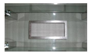
Place the burner over the buffer plate and drop into the glass cutout so it rests flush with the glass base.
